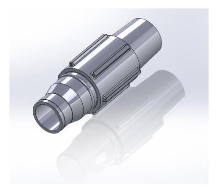
The above component, a 25 cm long piece (10 inches), was a flexible polymer over-molded onto a brass insert, and required a central mold core to orient and hold that brass piece during the molding process.
