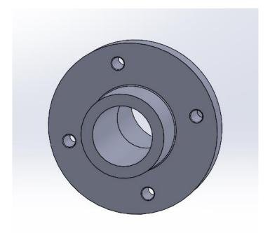
This component was a rigid material with a built-in mounting flange, also insert-molded with a brass piece with a central core in the mold to orient and hold that brass piece during the molding process.
